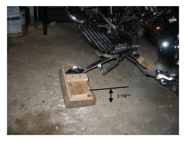
$\underline{\text{NOTE:}}$  This dimension may not be correct for 2004 models as the 2005 models have a different kickstand – the 2004 model will likely be thicker.
