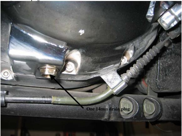
This plug drains the clutch area, not much oil comes out of this one if you drain the other two 17mm drains first. This plug is accessed from the left side of the motorcycle just behind the heal shifter. It has a small O-ring for a seal that should come off with the bolt don't lose it or you'll have to go get another one. Clean the sealing surface with a rag like you did for the 17mm drain plugs. Take care to just snug this bolt – over-torque can strip the threads.
