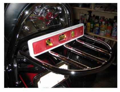
To be sure your blocks are the correct thickness the first time, lay a level across the luggage rack as shown. You may need to shim them slightly to hold the bike dead level.
